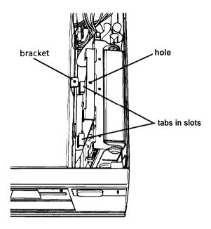
As shown above, fit the tabs on the mounting plate into the slots on the side of the subassembly. Then tilt the drive toward the subassembly and align the retaining screw hole on the mounting plate with the hole in the bracket.
